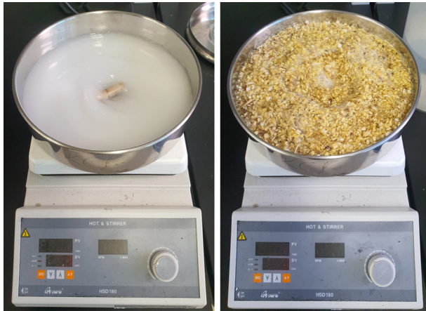
Fig. 6. Picture of kenaf+CaO sample stirring
