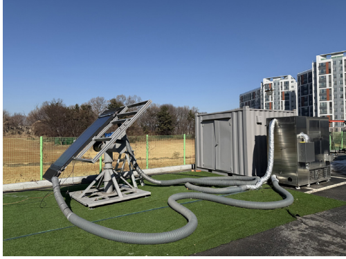
Fig. 5. Standard performance test of air-type PVT collector
