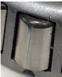
(c) Roller fault
