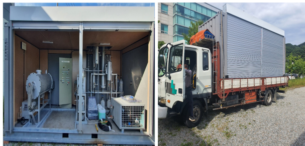
Fig. 5. Waste forest biomass transportable pyrolysis system
