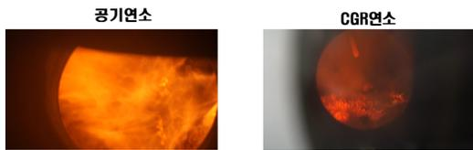
Fig. 7. Flames conditions at air incineration (left) & CGR incineration (right)
