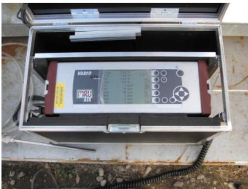
Fig. 4. VarioPlus analyzer
