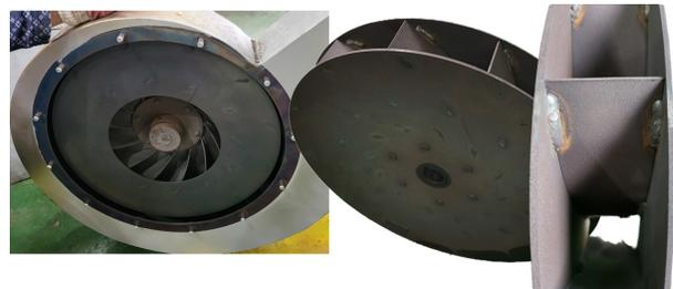
Fig. 6. Blower casing and impeller for CGR after temperature change test
