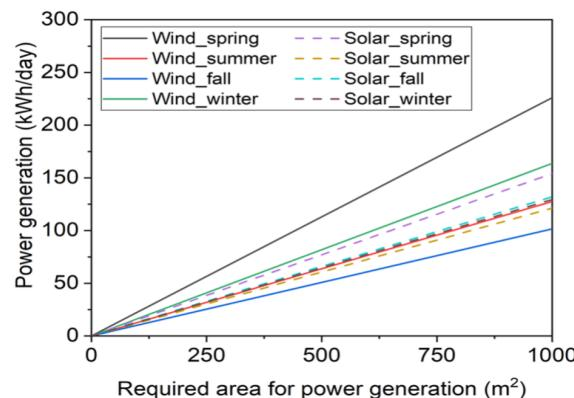
Fig. 6. Wind and solar power and required area for power generation at different seasons
