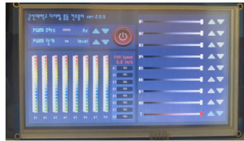
Fig. 7. PWM control system of the new digital wind tunnel
