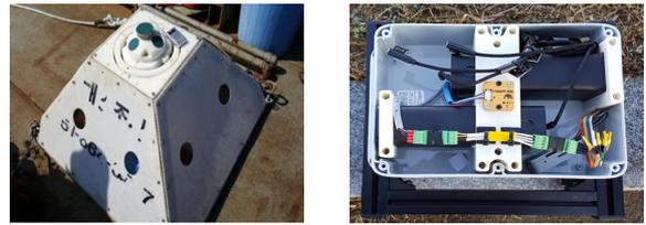
Fig. 4. Wave gauge and data recording system
