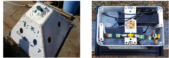
Fig. 4. Wave gauge and data recording system
