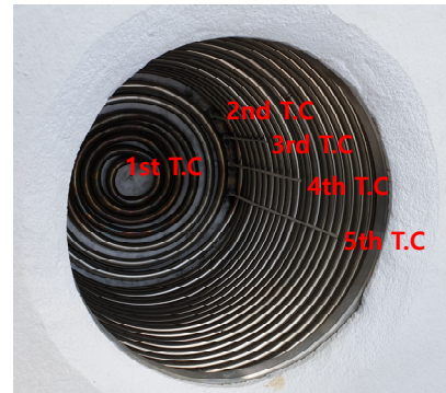
Fig. 7. Reactor(2) inside and temperature sensors
