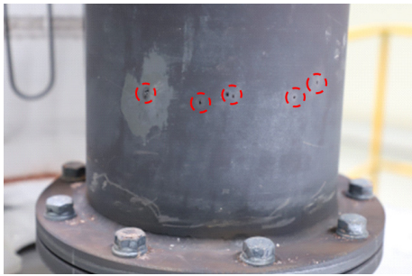
Fig. 17. Damaged reactor(4) (after experiment)
