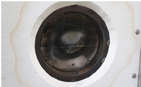
Fig. 6. Quartz window of reactor(1) (after experiment)
