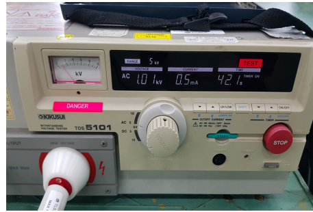
(b) Withstand voltage applied
