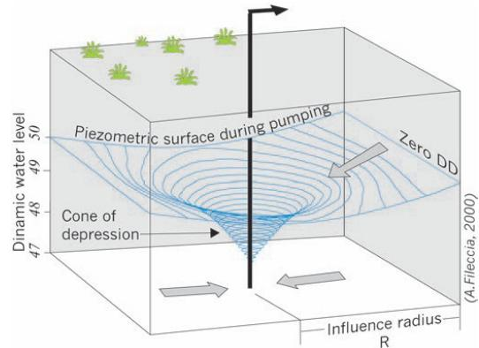
Fig. 1. Depression cone for a confined, homogeneous, isotropic aquifer with flat initial piezometric level and a fully penetrating well, without well bore storage<sup>[6]</sup>
