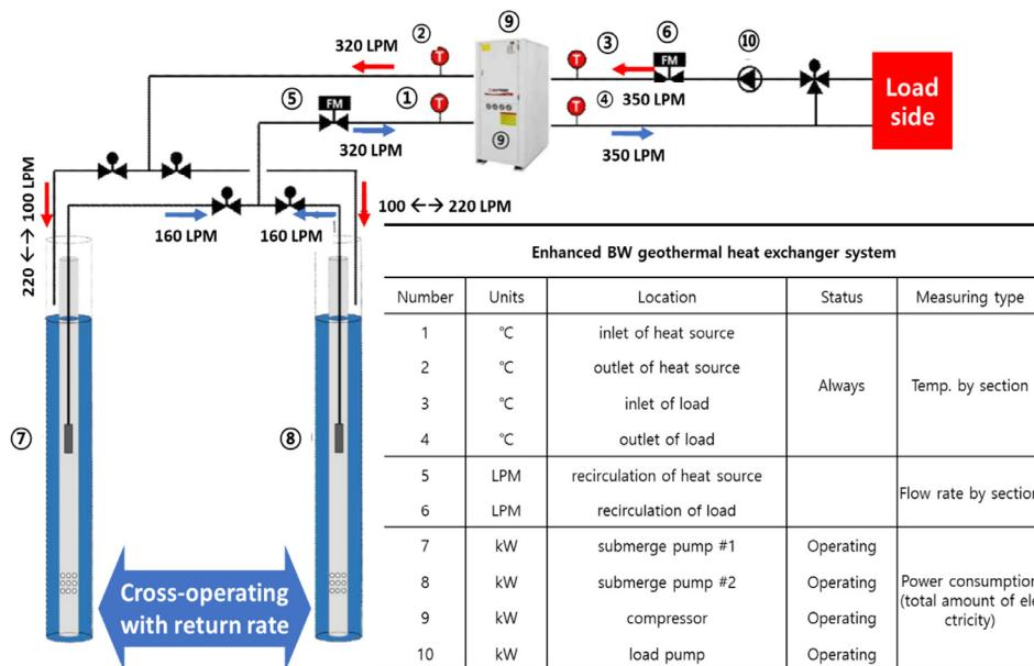
Fig. 5. System overview for calculating performance coefficients
