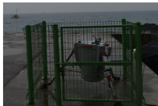
Fig. 9. Fixed LiDAR away from floating LiDAR system (distance 300 m)
