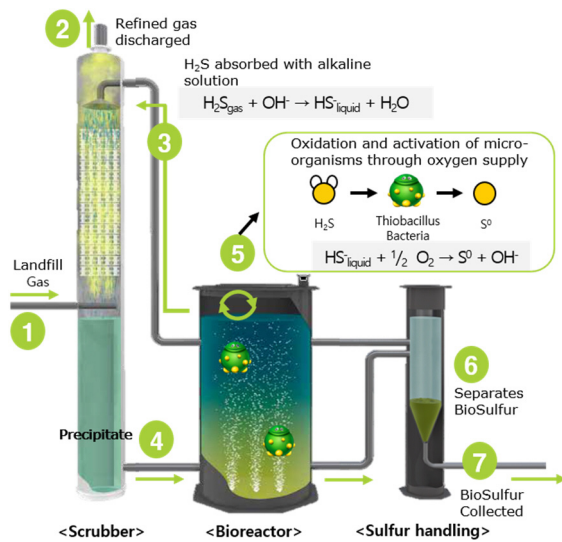
Fig. 2. THIOPAQ ® process diagram for the H 2 S removal from LFG
