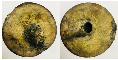
Fig. 2. Cross sections of Dike bamboo (Left : Bottom, Right : Top)
