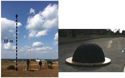
Fig. 3. 10 m mobile mat-mast (left) and microphone with secondary wind screen (right)
