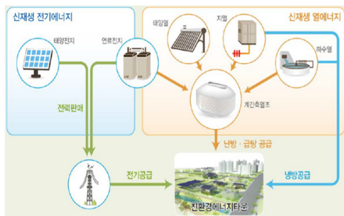
Fig. 1. Renewable heat supply based on seasonal thermal energy storage
