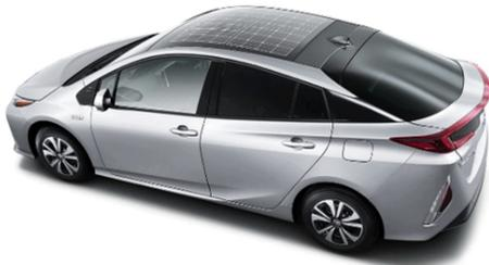
Fig. 2. New solar roof option for the 2017 Prius Prime developed by Panasonic
