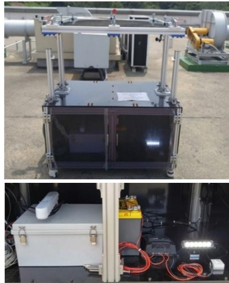
Fig. 5. Monitoring system used in outdoor testing for developed a-Si:H single-junction PV module
