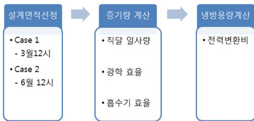
Fig. 5. solar thermal cooling model analysis model
