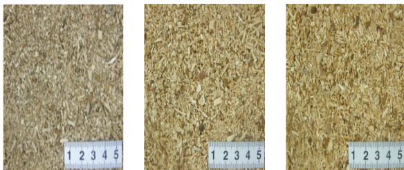
Fig. 1. Images of mongolian oak (left), pitch pine (middle) and larch (right) sawdust used for the production of wood pellets
