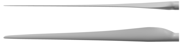
Fig. 1. Illustration of DSB48.3, a 3-MW wind turbine blade designed for IEC wind class IIA
